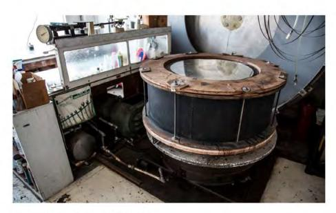
[Fig. B] Centrifugal vertical spincasting mold tool (diam. 40 in.), 1971. Eversley reused a 1936 turntable to create this tool to produce his parabolic sculptures.
